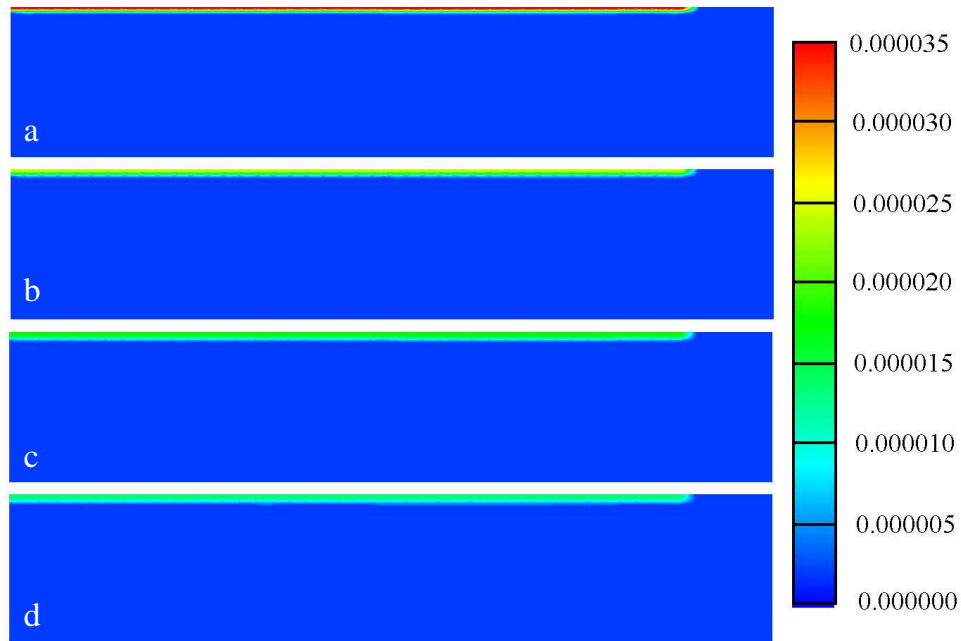
Figure 4.8: Concentration profiles of ammonium ( \text{mg}/\text{cm}^3 ) for scenario A at (a) 3 months, (b) 6 months, (c) 9 months, and (d) 12 months. Note that the vertical axis has been exaggerated by a factor of 3.
